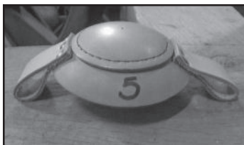
A Big-Wilf muffle, tailor made for St Edmund's No 5 bell clapper
